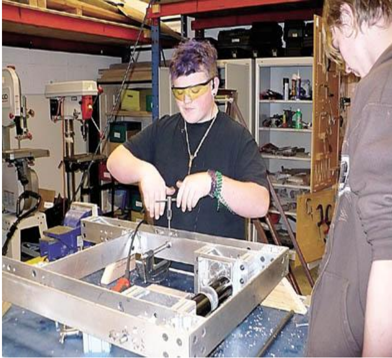
Tech High Robotics member Ian Collins taps and threads holes for the school's new robot as Quest Meyer looks on.
